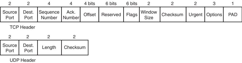
Figure 31-7 TCP and UDP Headers
