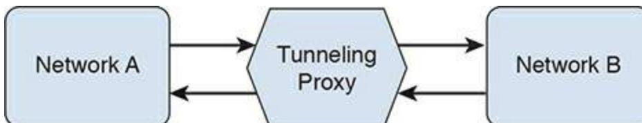
**Figure 21-6** Tunneling Proxy
