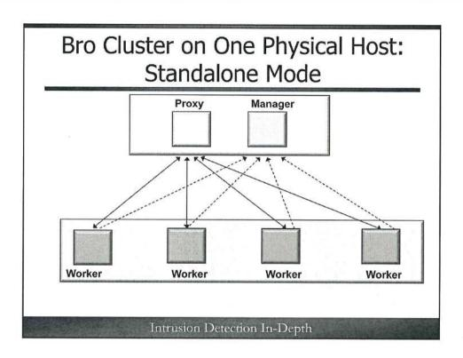
Bro is very flexible in its configuration options, facilitating capacity planning and scaling. The simplest, though least flexible option, is to put a Bro cluster on one physical host more commonly known as a standalone implementation. There is a single proxy, a single manager, and one or more workers that are manifested as distinct processes on the host.
