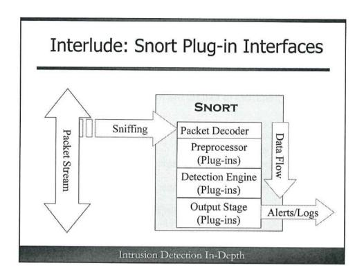
This slide shows the way packets travel through Snort and are processed by the three types of plug-ins. The packets are captured from the network interface. There is a high level packet decoder that identifies the various layers found in the packet.
