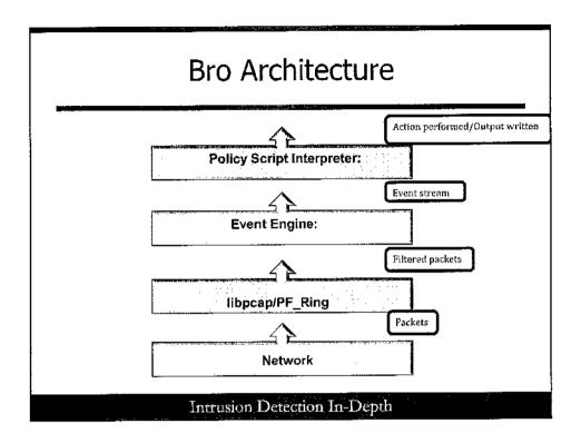
Bro's architecture relies on libpcap at its base to sniff and filter packets much like Snort. PF\_RING can be wrapped around libpcap when there are multiple Bro sniffing processes on a single host, permitting the traffic to be directed to individual cores on multi-core architecture hosts. Think of it as host load balancing.
