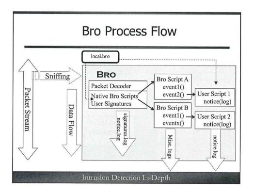
This slide shows the way Bro processes traffic. Bro decodes the packet and invokes some native scripts that analyze and process the packet protocols much the way Snort preprocessors do. While simple signatures can be written by the user, Bro includes none. The native Bro scripts consist of code and logic and they define events. Events are a very important part of Bro.
