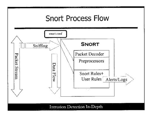
This slide shows how Snort processes traffic. The traffic is sniffed from the network interface and passed to Snort. The packet is decoded and then different preprocessors prepare the traffic to be examined by the rules by reassembling streams, and parsing the embedded protocols, for instance. Then rules that come with Snort and any user-supplied rules examine the traffic for noteworthy activity. The packets and alerts associated with this activity are placed in alert and log files.
