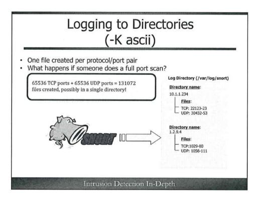
Here's an example of how Snort's "-K ascii" logging mechanism works. Snort, by default, logs to "/var/log/snort" unless otherwise specified with the -l name command line switch, identifying a log directory that must already exist. When packets come in, a subdirectory in the log directory is created for the relevant source IP address if it doesn't already exists. Then files containing the packet dumps are created within that directory based on the protocol and ports.
