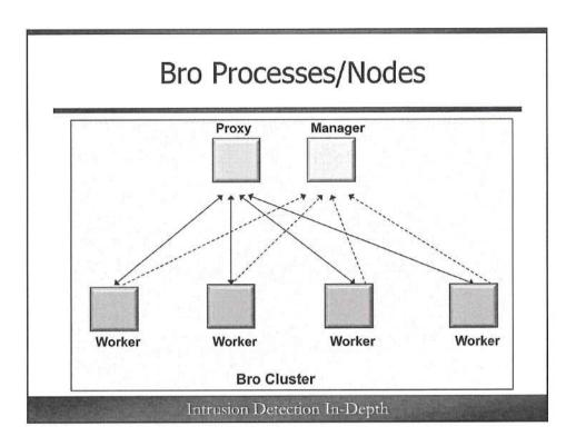
Bro has three different functional nodes – the worker, the manager, and the proxy. Together these three nodes form what is known as a Bro cluster. Bro even has its own communications protocol to transmit Bro traffic between nodes.
