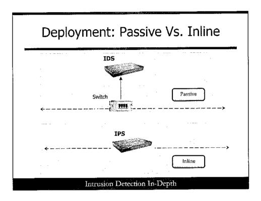
Snort can be deployed as a passive sniffing sensor that alerts and logs noteworthy traffic. This is the default mode. Another option is inline where traffic actually traverses two interfaces of the Snort box. This method allows traffic to be blocked, optionally.
