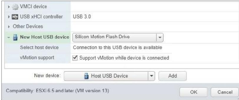
**FIGURE 11.25** USB enabled for vMotion
