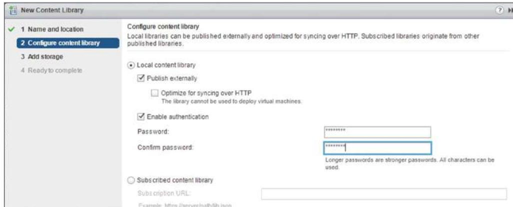
When configuring local storage (see Figure 11.30), note that SMB only works with Windows-installed vCenter servers. While a VCSA server will allow you to choose SMB, it will never connect to the share and will use local storage on the appliance for the library.
