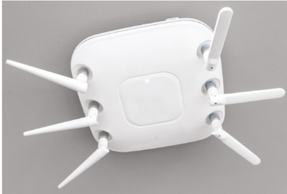
FIGURE 16.6 A wireless access point (WAP)
