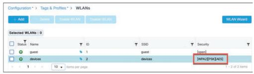
**Figure 20-5** *Verifying PSK Authentication from the List of WLANs*
