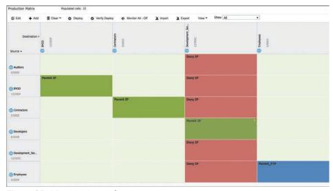
Figure 25-14 SGACL Production Matrix View
