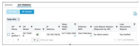
Figure 21-13 Displaying AP Join Statistics
