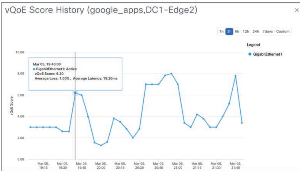
Figure 12-23 vQoE Score History on the DC1-Edge2 Router (Gateway)
