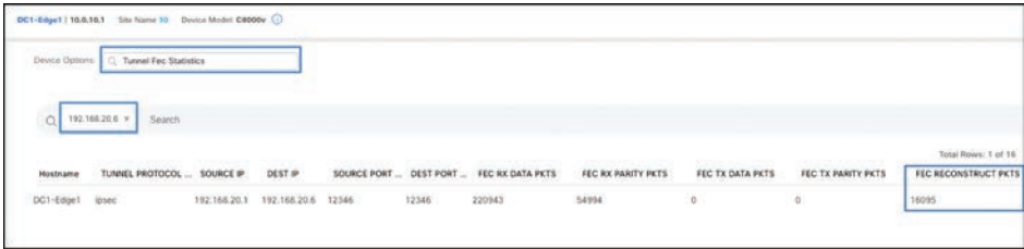
Figure 8-55 The Current FEC Reconstructs Packets
