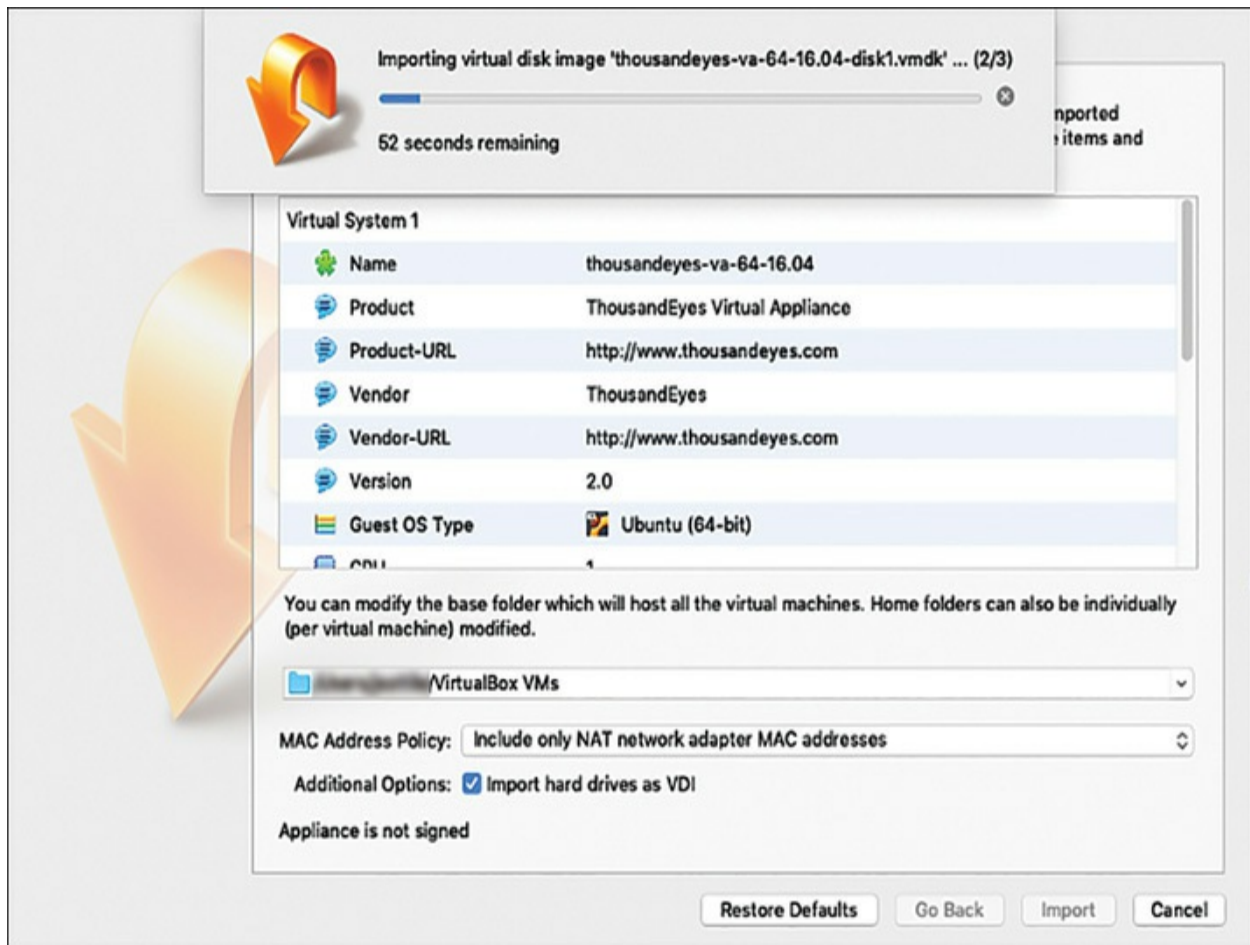
Figure 2-6 Installing a New VM Enterprise Agent
