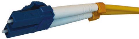
FIGURE 3.9 A sample LC fiber-optic connector
