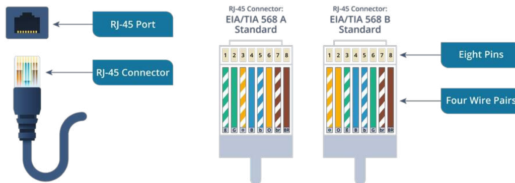
T568A and T568B wiring diagrams. (Images © 123RF.com.)
