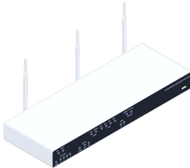
An integrated services router. This type of device combines DSL Internet access with Ethernet switch, Wi-Fi, and VoIP for a "one box" solution for remote sites and branch offices. (Image © 123RF.com.)
