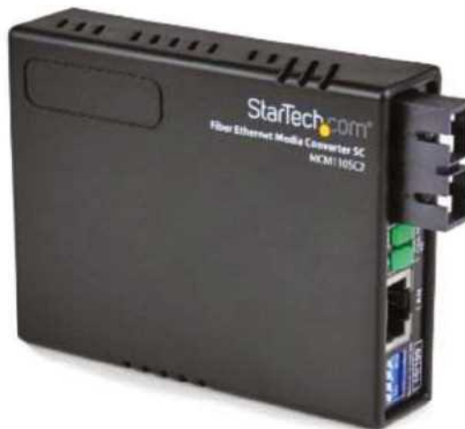
FIGURE 3.14 Multimode fiber to Ethernet
