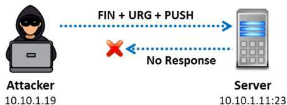
Figure 3.46: Xmas scan when the port is open
