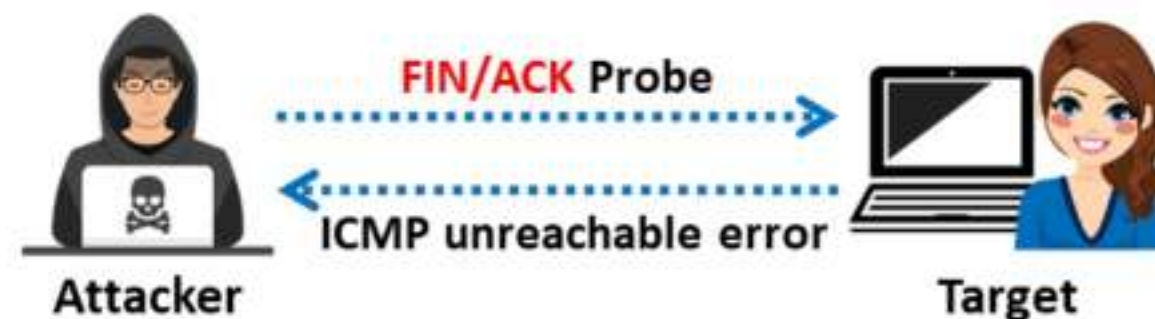
Figure 3.51: TCP Maimon scan result of filtered port
