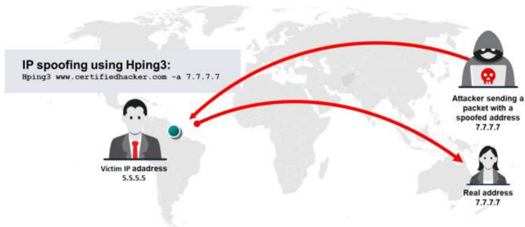
Figure 3.111: IP Spoofing using Hping3
