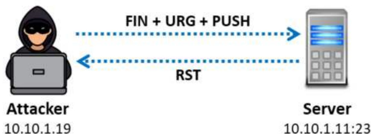
Figure 3.46: Xmas scan when the port is open
