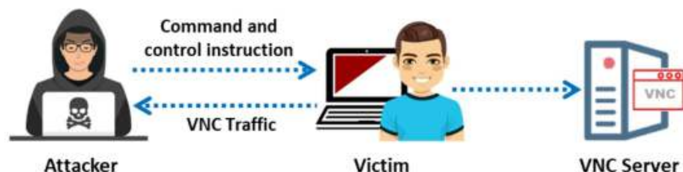
Figure 7.19: Working of VNC Trojan
