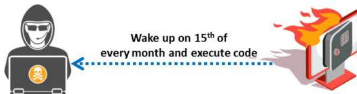
Figure 7.46: Working of sparse infector virus
