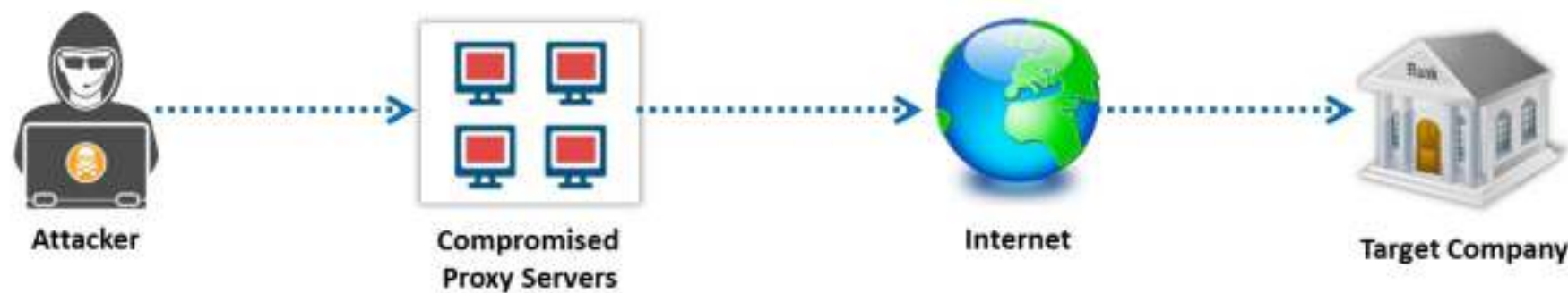
Figure 7.35: Propagating and deploying Trojan through proxy servers
