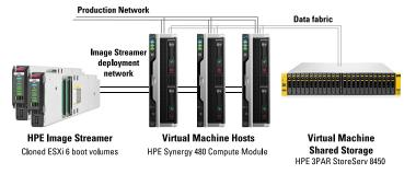
Figure 5-3: Stateless virtualization deployment architecture with Image Streamer.
