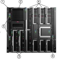
Figure 3-1: The front of the HPE Synergy frame.
