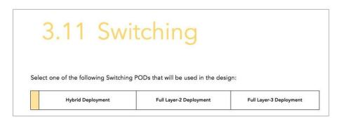
Great, now here we need to determine which Switching deployment will be used among the LAN POD. This can be a hybrid, full Layer-2, or full Layer-3 deployment. It is important to look at each POD to determine which one will align with the business requirements and match your preference as the network architect/engineer. If you remember the example I gave in the beginning, if you want minimal layer-2 then you might choose the "Full Layer-3 Deployment" POD.
