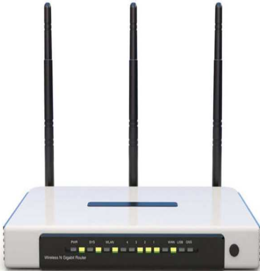
Figure 36-5 LED Lights on a Wireless Router
