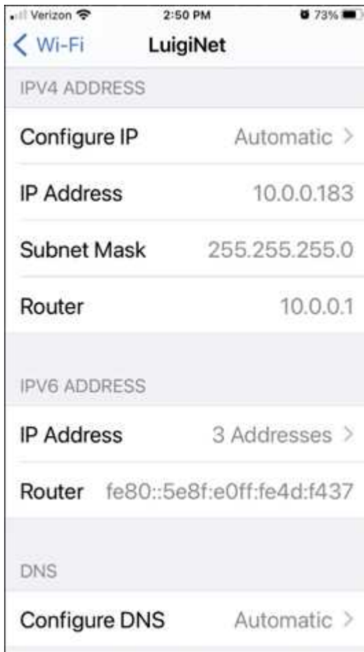
Figure 37-35 Verifying the Wireless Setting in iOS
