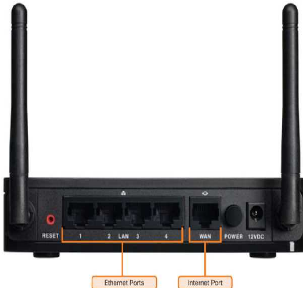
Figure 4-2 Back Panel of a Home Wireless Router
