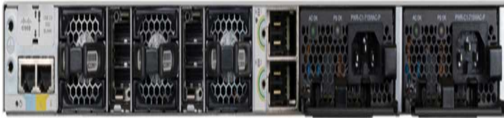
Figure 35-15 Back Panel of the Cisco Catalyst 9300 48S
