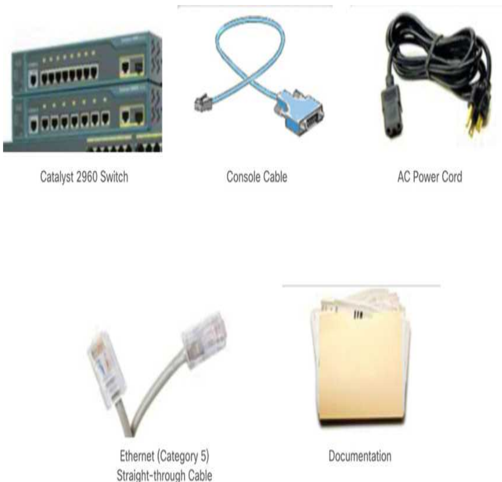
Figure 35-13 Components for Connecting to a Switch
