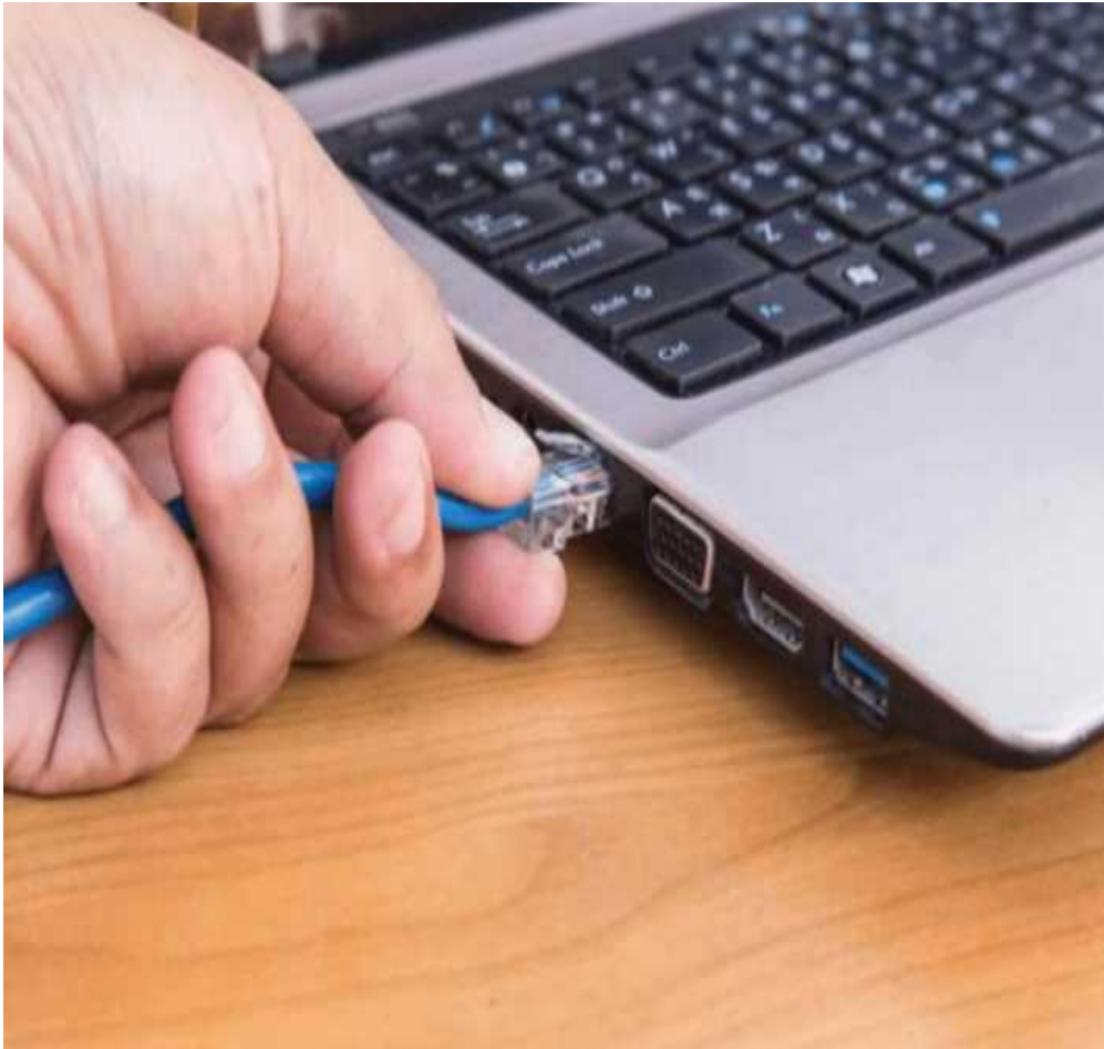
Figure 30-3 Wired Connection Using an Ethernet NIC
