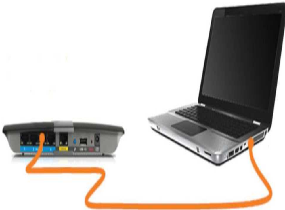
Figure 30-2 Wired Connection to a Wireless Router
