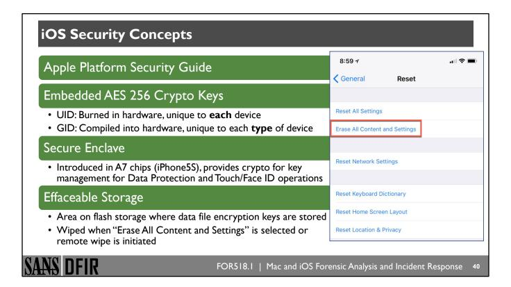
Cryptographic keys are burned or compiled into the physical hardware of the device. The Secure Enclave coprocessor provides the cryptographic processing using these keys for file system encryption and Data Protection, as well as usage of Touch ID. The Secure Enclave was introduced in the A7 chips in the iPhone 5S generation of devices.
