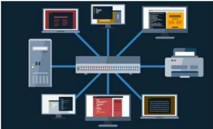
The benefit of the star topology is that it is easy to maintain, any computer or cable in the network could fail, and the others would not be affected. Of course, if the central point fails then that is a different story.
