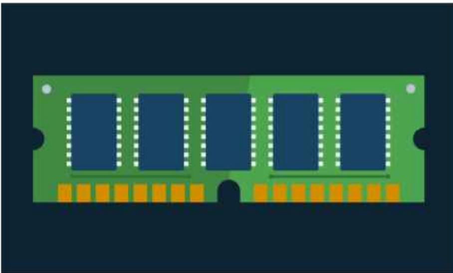
Here we have a 'stick' of RAM. The gold connector at the bottom of the RAM 'stick' slots into the RAM slots on the motherboard. The 'stick' in the image above is 8GB of RAM. Think of RAM as the number of things you can have open on your computer at once. So with 8GB of RAM, you can have 8GB of software running all at once. Part of that will be taken up with the operating system (e.g. Windows), but the rest will be for whichever programs, images etc. you have open at once.
