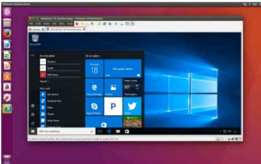
Here we have a Linux system running VMware (a popular virtualization software); the operating system inside the virtual machine is Windows 10.
