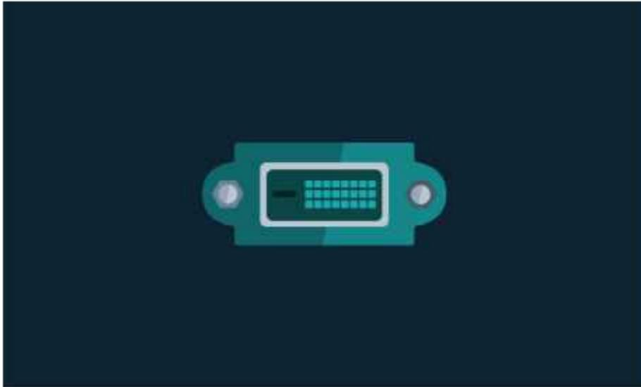
Once again, note the area for two thumb screws which need to be tightened after the connection is plugged in.
