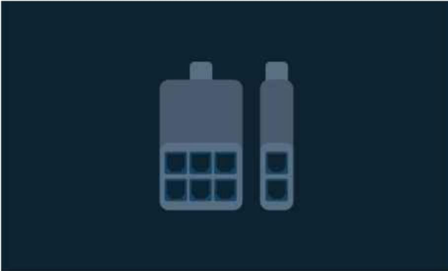
The above image shows a PCI-E power connector, which usually runs to a graphics card. Again, some cards need six pins and some need eight, and therefore you will commonly find cables with an optional extra two pins.
