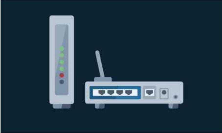
Note that most routers these days include the functionality of a switch, but the number of ports they offer is limited. If you need more ports, you can buy a switch and plug it into one of the LAN ports on the router.
