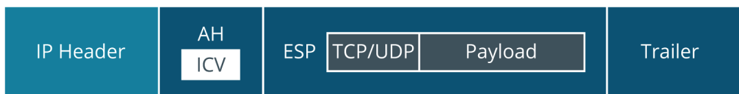
IPSec datagram using AH and ESP in transport mode.
