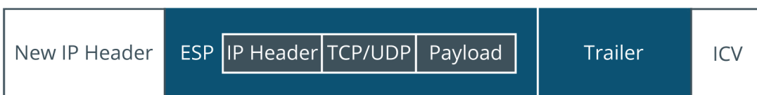
IPSec datagram using ESP in tunnel mode.
