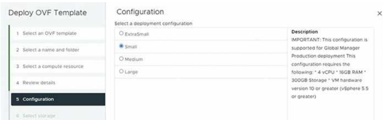
Figure 13.6: Selecting size of Global Manager appliance
