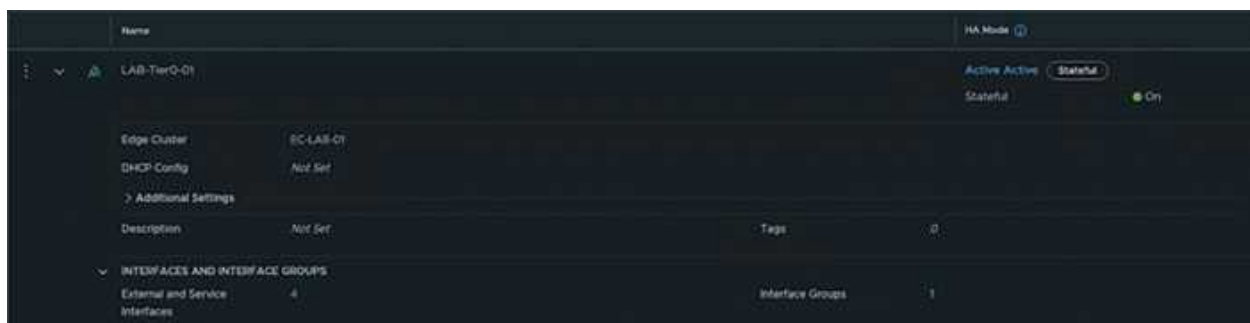
Figure 11.8: Viewing a Tier0 gateway running in stateful Active-Active HA
