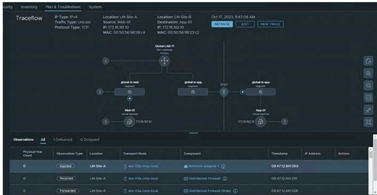
Figure 13.68: Running Traceflow from NSX Global Manager
