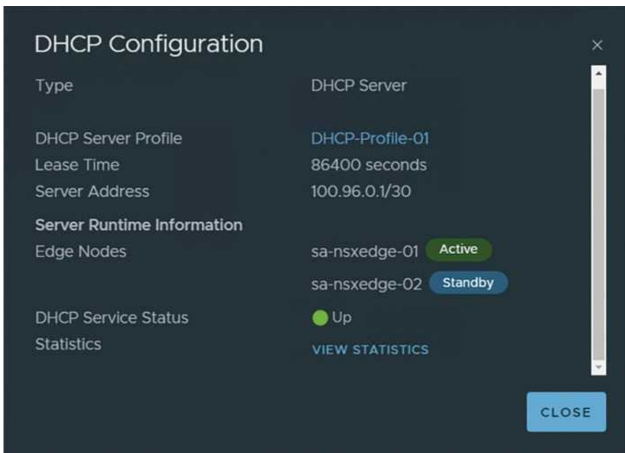
Figure 11.40: Viewing DHCP Configuration on NSX gateway
