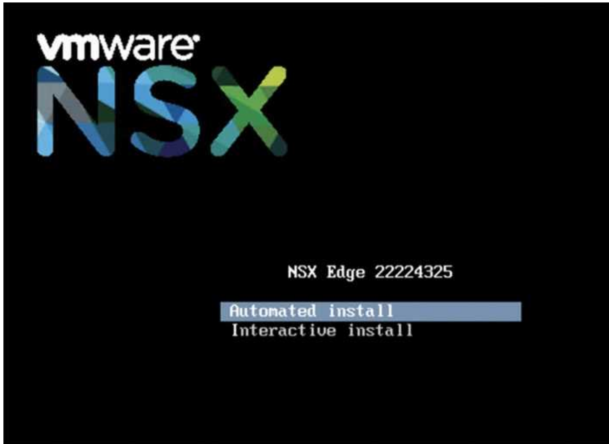
Figure 4.25: Booting physical server with NSX Edge ISO
