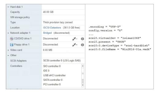
FIGURE 11.11 GUI and .vmx file for a VM with a SCSI drive
