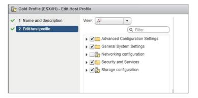
Once the profile contains the settings desired you can attach it to individual hosts or all hosts in a cluster by using the Attach/Detach wizard in Host Profiles or the Host Profiles actions menu available from a cluster or host object (Figure 9.19). Be advised that you can only attach one profile to a host at a time.
