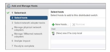
4. On the Select Network Adapter Tasks screen, select Manage Physical Adapters.
