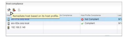
If you no longer wish to associate a host profile with a particular host or all the hosts in a cluster, you can detach the profile using the Action menu on the host or cluster object (Figure 9.24) or from within the host profile.
