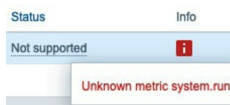
Figure 3.84 – Unsupported item information, Unknown metric system.run
