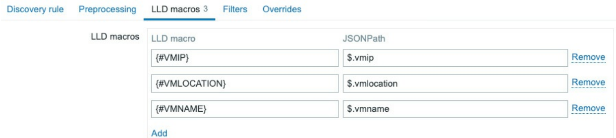
Figure 7.66 – The Zabbix LLD macros tab for the hosts.from.json LLD rule
