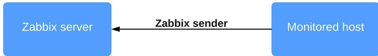
Figure 3.40 – Zabbix server trap receiver diagram
