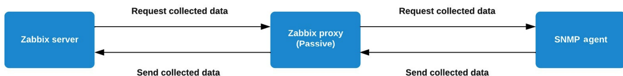
Figure 8.15 – A completely passive Zabbix setup with proxy
