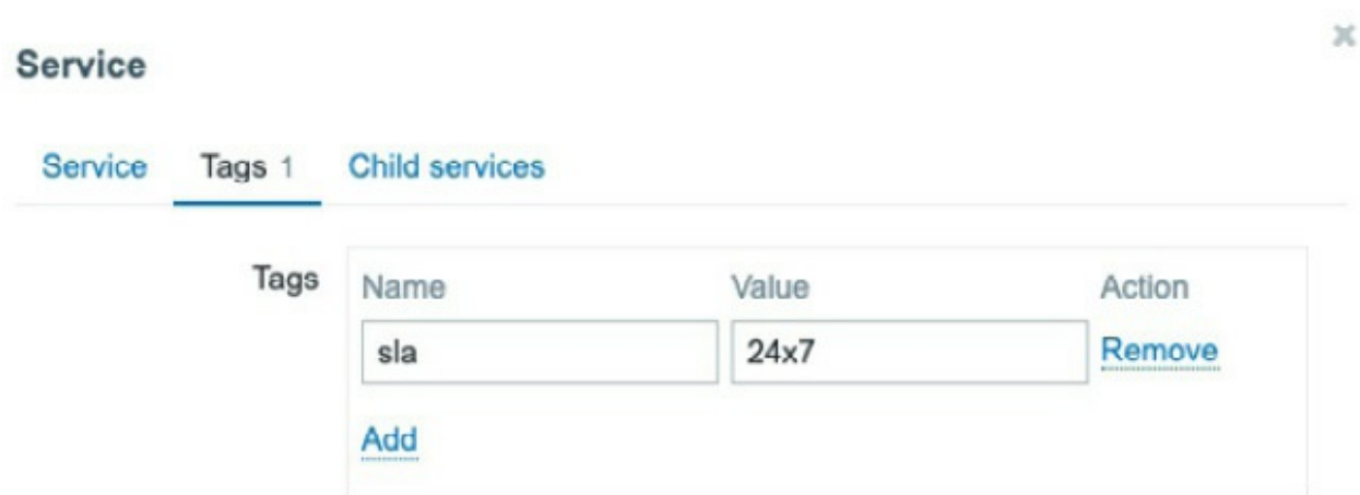
Figure 6.97 – Service | Service – Zabbix database service – the Tags tab
