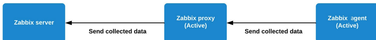
Figure 8.16 – A completely active Zabbix setup with proxy
